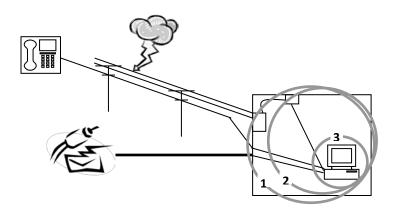
The zones of protection approach is designed to control surges at their initial point of entry or reduce them to a level that can be controlled at the next stage
