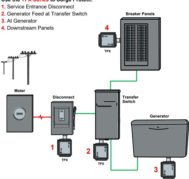
**Note:** Additional surge protection can be placed on the output of the transfer switch. This is done when the transfer switch is placed outside and is at risk of surges from lightning.
