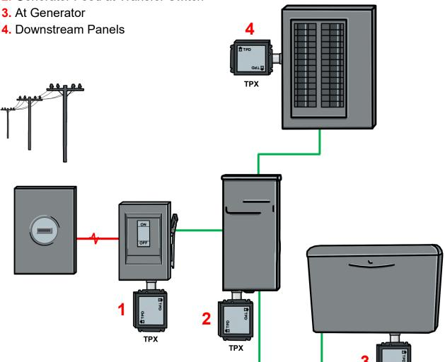
**Note:** Additional surge protection can be placed on the output of the transfer switch. This is done when the transfer switch is placed outside and is at risk of surges from lightning.
