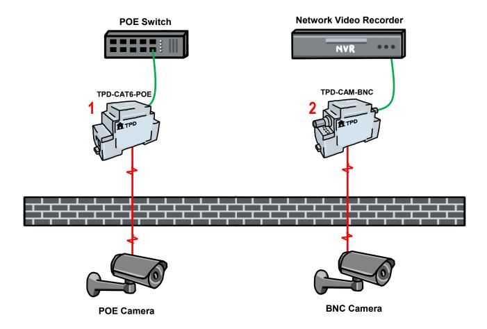
Note: For analog cameras with F connections use TPD-CAM-BNC-F
