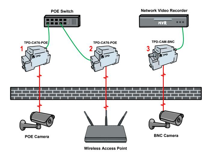
Note: For analog cameras with F connections use TPD-CAM-BNC-F
